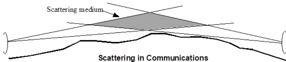
Figure 1. Over-the-horizon contacts made by radio amateurs usually involve scattering.
