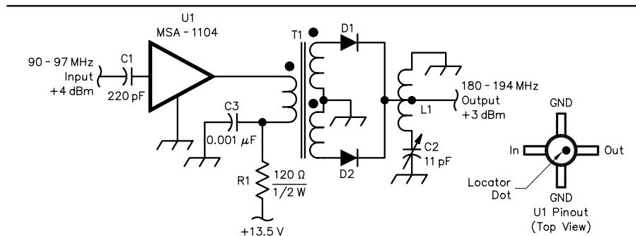
Fig 4—Frequency doubler schematic.
